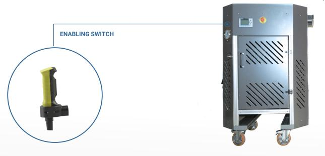
The automatic MK45-3000NX Powerpack was designed to operate at factory with a high number of hydraulic tensioner.
